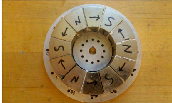
Fig. 8 Rotor disk with Halbach array.
